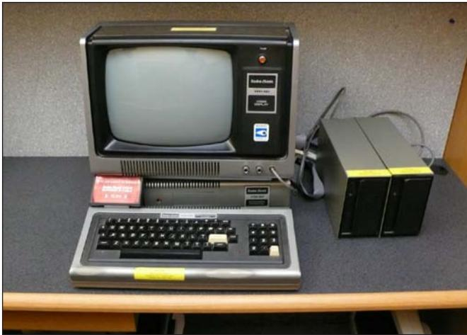
Figure 2. An early microcomputer TRS-80 platform with memory storage consisting of two 5 1/4" floppy drives.
