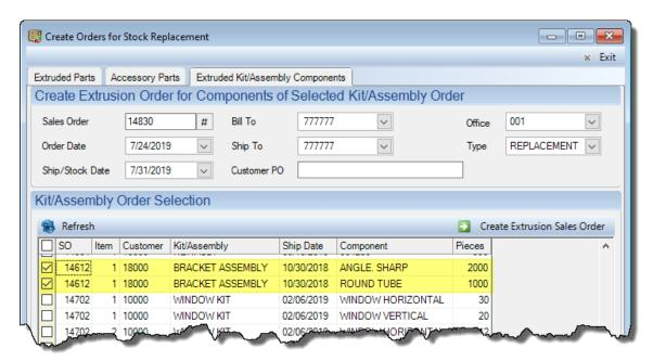
In the screen-shot above, the assembly named "Bracket Assembly" requires two extruded components. Simply click the SO number, and all components for the assembly are selected. Then click Create Extrusion Sales Order to get these component jobs underway. This is done on the new Extruded Kit/Assembly Components tab of the Stock Replacement screen.
