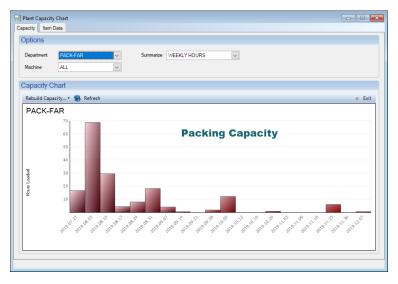
You can quickly configure EPICS to determine the effective capacity for each production department and machine in the plant. Then, using data from all open sales orders, reserves, and unposted orders, the Capacity Planning Module calculates the time required to complete each job. Subtracting these from the
